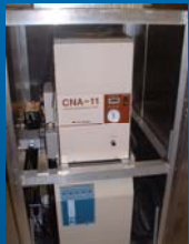
Figure 1 Bottom row of images shows our superconducting gravimeter (SG) system. The gravimeter and associated instruments are contained within two enclosures, which have cooling systems and waterproof aluminum boxes. The hand-lift helps to transport and install the system in the field. By making the instrument transportable, one may choose sites where better-defined hydrologic problems can be investigated, and consider tectonic, volcanic, and other applications, such as deep slow earthquakes (Crossley D. et. al., 1999). The lower row of images shows from left to right: Power Supply and 4 Kelvin refrigerator in one enclosure; 35 liter helium dewar containing sensor in the gravimeter enclosure, with instrument rack on right; and right, the instrument rack showing GWR data logger, volt meter, barometer, electronics, and at the right side, the enclosure heating / cooling system.
